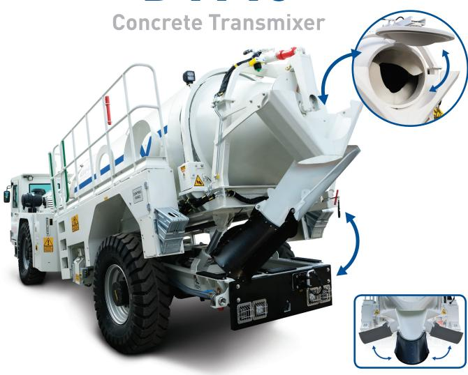
• Hydraullically controlled shuter and chute - Drum tilt up to 130
